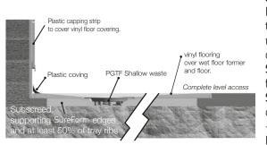
**Step 1.** Position the SureForm over the desired location for the shower. Formers are trimmable and can be cut to down to minimum 150mm to the waste area. Ensure the cut edges are straight and put towards the wall mounted side. If necessary cut to the correct size with a suitable circular saw or a fine toothed blade. Mark around the edge of the shower former.
