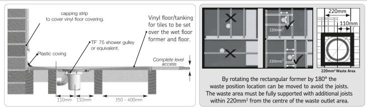
**Step 1.** Position the SureForm over the desired location for the shower and mark around the edge of the shower former. Align the SureForm into position and check for waste outlet entry. To avoid or minimise joist overlap, the SureForm former waste location is offset and it can be rotated 180° to allow the waste to fit between the joists.
